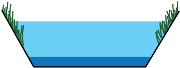
Conventional trapezoidal-shaped channel
